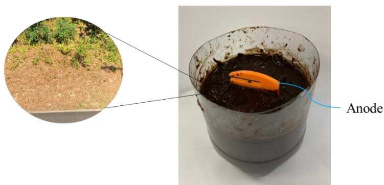
Figure 2. Method of biofilm formation on anode surfaces.
