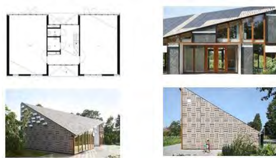
Figure 10: (Left-Top) the cross-ventilation where there are openings in the opposite sides of the building – (Right- Top) the solar panels, (Left – Bottom) birdhouses, (Right – Bottom) nook (Wang, 2015)
