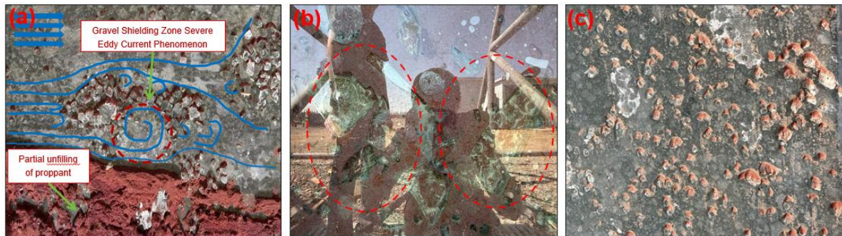
Figure 3. Fluid and particle characteristics within fractures. (a) Schematic illustrating changes in flow regime through the gravel zone; (b) Non-uniform distribution of proppants; (c) Aggregation of proppants in the upper gravel section.
