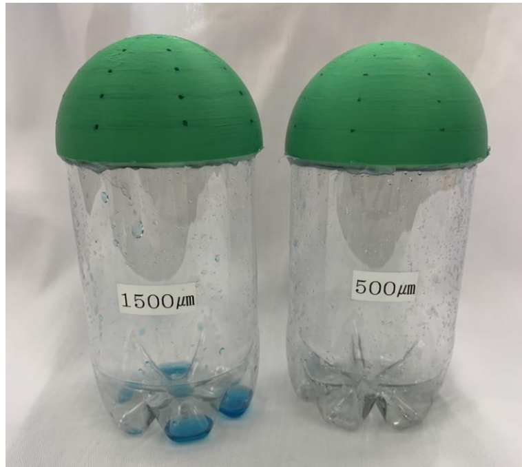
Figure 8. Comparison of the effectiveness of cathodic protection by the size of holes in the upper ball-shaped cover.
