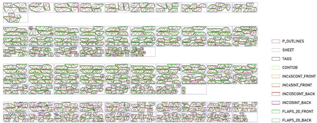
Figure 5. Final nesting of the panels. Layer naming according to the typology of the milling process, figure reproduced from ACADIA 2024 Project Paper “Form Freed”. (2020, WOOD-SKIN®).
