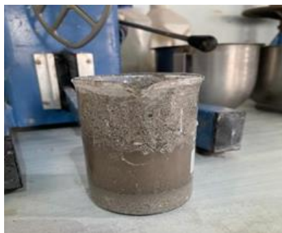
Figure 2: Absorption test for the used PCB
