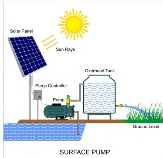
Figure 3. Solar power water pump (Source: Nicholls, 2006).
