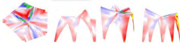
Figure 6. Karamba structural analysis showing areas of compression (Red), tension (Blue), maximum tension (green), maximum compression (yellow), and neutral areas (white).
