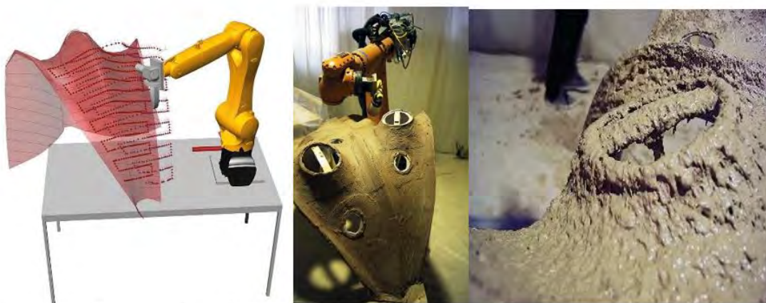
Figure 10. (a) Kuka PRC simulation of robotic trajectories after the first scan of the temporary formwork. (b) Middle layers of clay mix containing fibers applied by robotic spraying. (c) Close-up of the freshly projected fibrous clay mix robotically applied on the shell.
