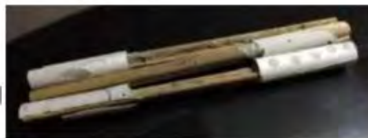
Figure 19. Longitudinal cracks in Epoxy and Specimen (Author's own, n.d.)
