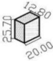
Figure 27. Dimensions of the specimen of compression (Author's own, n.d.)
