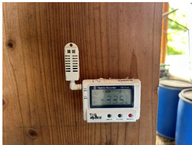
Figure 5. A temperature and humidity data logger used for field measurements.
