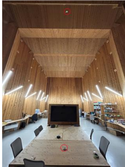
Figure 3. Indoor measurement point layout in the CLT office building.
