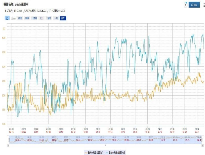
Figure 4. An Online monitoring platform showing real-time temperature and humidity data.
