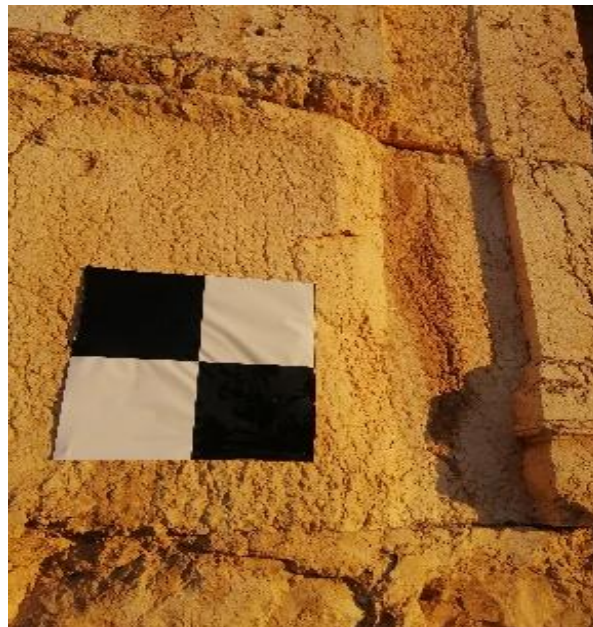
Figure 5. Example of one of the 27 control points attached to the wall (Source: Author, 2025).
