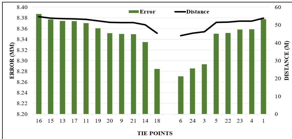
Figure 8. The distribution diagram of the relative errors of points coordinates depending on the distances to the laser scanning station (surveyed from station №. 7) (Source: Author, 2025).
