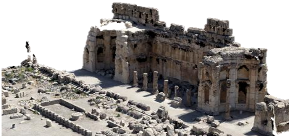
Figure 9. A point cloud model derived from a survey using a UAV (Source: Author, 2025).
