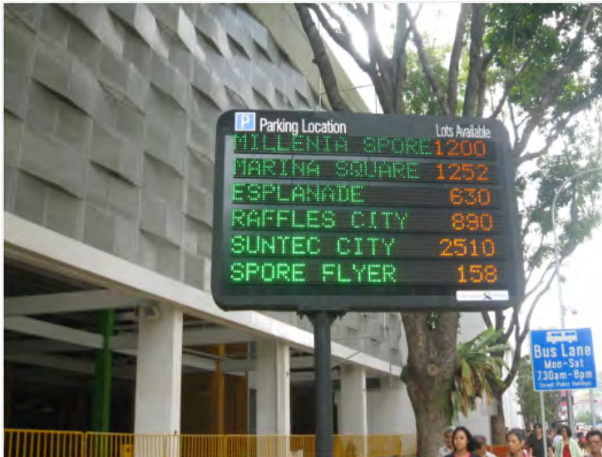
Figure 4. A Parking Guidance System in Singapore (for example). (Harman, 2009)
