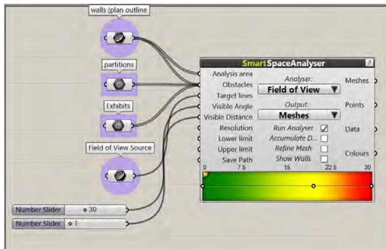
Figure 1. Field of view Component (Smart space analyzer)
