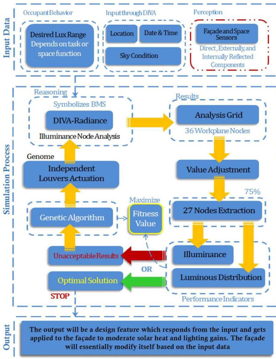
Figure 6. System logic – the path of data exchange between the proposed algorithm and the daylighting simulation tool. (El-Sheikh, 2011)
