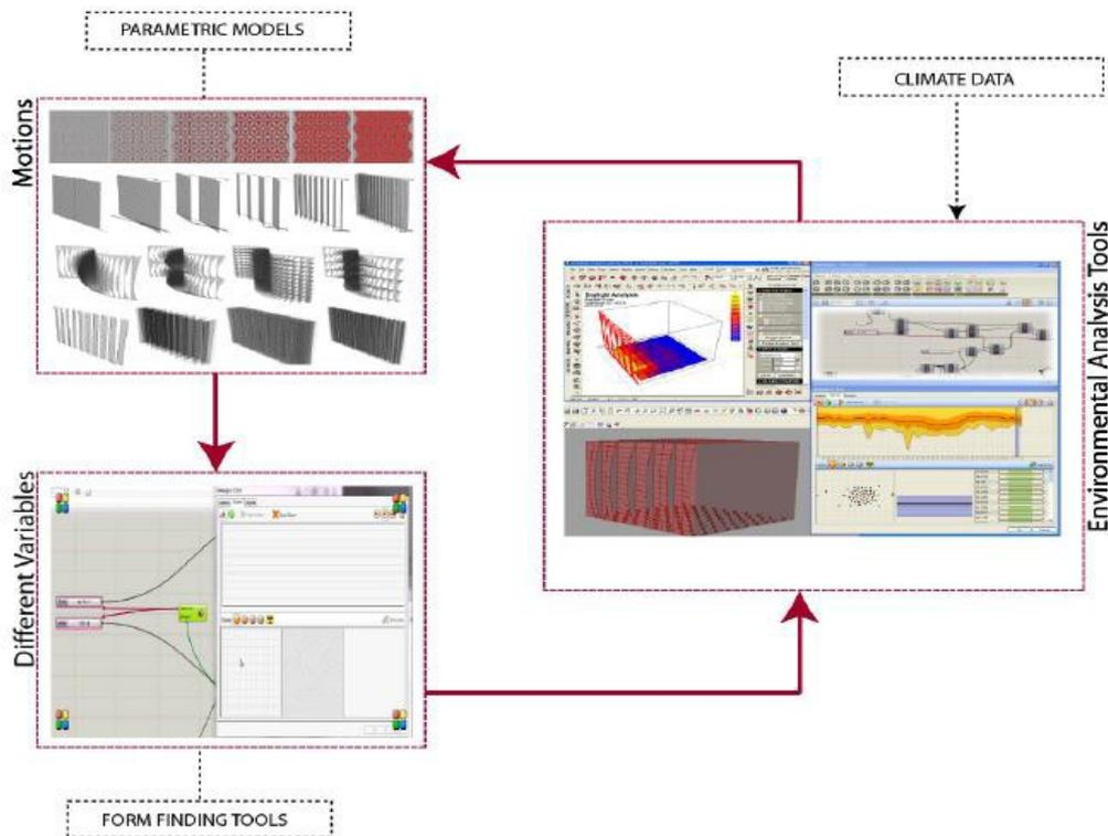
Figure 5. Explains the process of these simulations to find the optimal facades configuration. The variables were represented by sliders with set minimum and maximum values depending on designers' requirements (Cheung, 2013)
