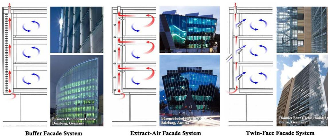
Figure 2. Examples of double façade types of buffer, twin face and extract-air, Source: Author
